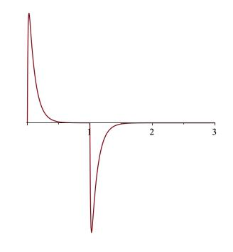
When the switch is closed at t = 0 the current spikes (clockwise) while the capacitor charges. When the switch is open at t = 1 the current spikes (anticlockwise) while the capacitor discharges.
