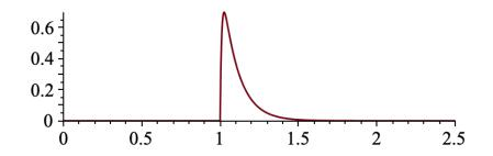
The current spikes when the switch is closed but returns quickly to zero. Interpretation: The battery causes current that charges the capacitor. When the capacitor is fully charged the current stops. In our case we had  $R^2 - 4L/C > 0$ . If  $R^2 - 4L/C < 0$  then the polynomial  $Ls^2 + Rs + 1/C$  has imaginary roots and the current will oscillate as it goes to zero.
