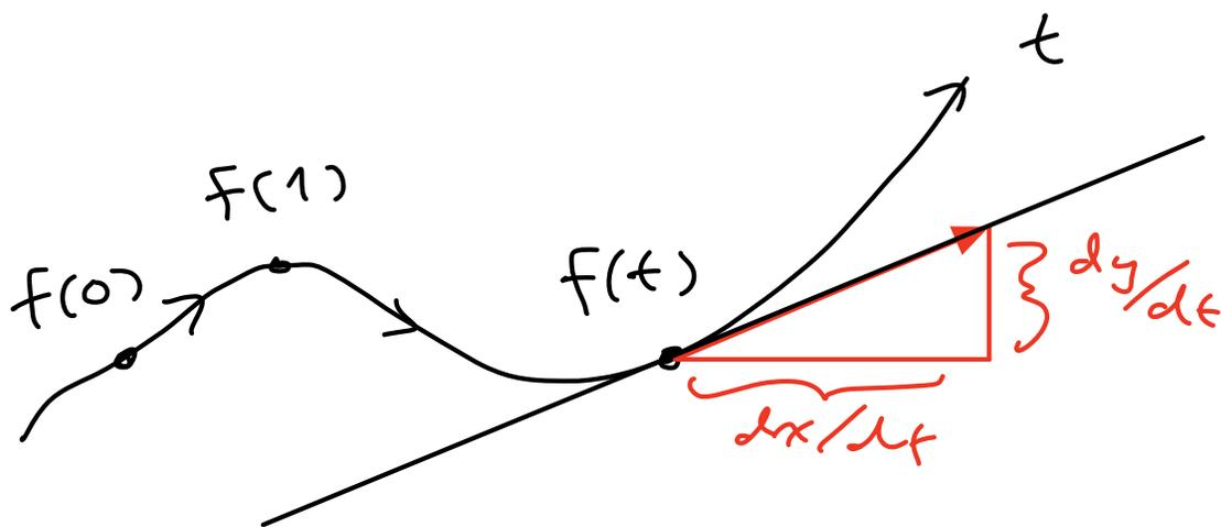
Picture: Velocity is tangent to the path. Hence the slope of the tangent line is
