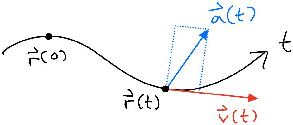
Strictly speaking: The acceleration has a component in the tangent direction that changes the speed & a component in a normal direction that causes curving.
