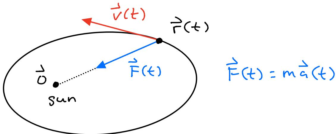
Problem : Given the initial position  $\vec{r}(0)$  & velocity  $\vec{v}(0)$ , compute the orbit  $\vec{r}(t) = \langle x(t), y(t), z(t) \rangle$ .
