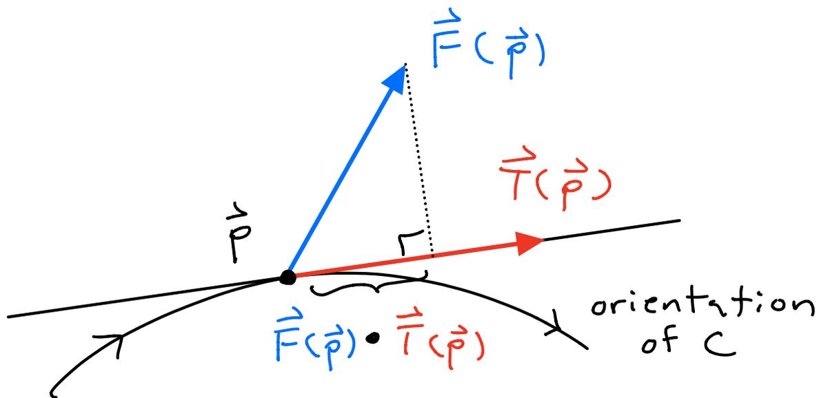
The component of the vector  $\vec{F}(\vec{p})$  in the direction of the tangent  $\vec{T}(\vec{p})$  is the dot product  $\vec{F}(\vec{p}) \cdot \vec{T}(\vec{p})$ ,
