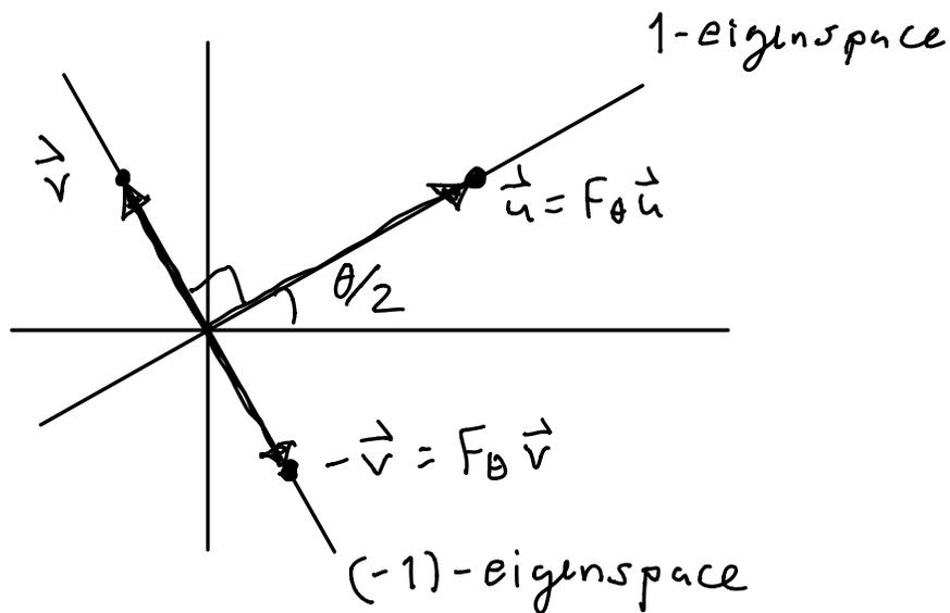
Also, for any vector  $\vec{v} \perp$  to the line we have  $F_\theta \vec{v} = -\vec{v} = (-1)\vec{v}$ .
