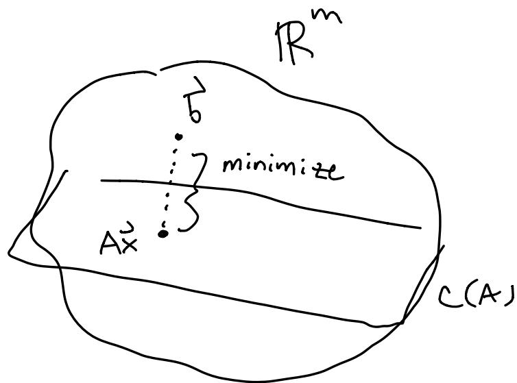
If  $\vec{b}$  is not in the column space, we want to find some point  $A\vec{x}$  in the column space such that the distance
