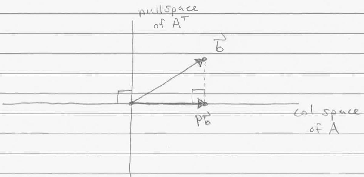
In the picture I have drawn a general vector  $\vec{b}$  and its projection  $P\vec{b}$  into the column space.
