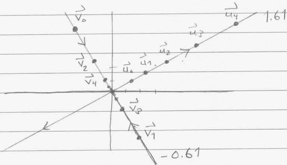
I have labeled each eigenline by its eigenvalue. The arrows indicate that one eigenline tends to expand ( $|\varphi_1| > 1$ ) while the other tends to contract ( $|\varphi_2| < 1$ ).
