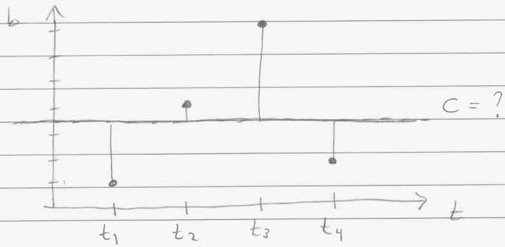
"Best" will mean that we minimize the sum of the squares of the vertical errors in the picture. To this we first naively try to find a horizontal line that contains all four points:
