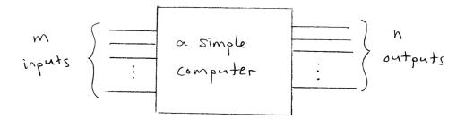
Each wire can only carry two signals: 0 (represented by low voltage) or 1 (represented by high voltage). Suppose that our computer is designed to add two numbers from the range 0 to 7. Using binary arithmetic, we could encode the input with 6 wires and the output with 4 wires. To compute "6 + 5" we would input 110101. Then the correct output would be 1011, which corresponds to "11". We will discuss the details in Section 2.4.
